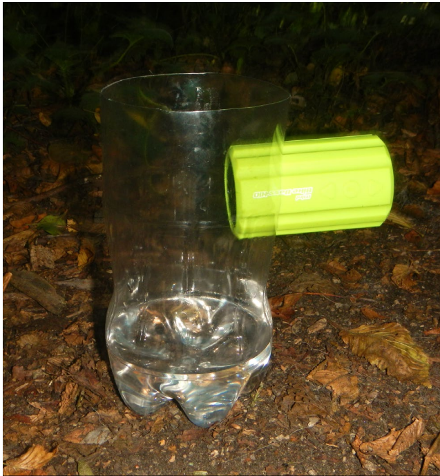
FIGURE 1 Acoustic “bottle trap” used for this study. Acoustic stimuli were broadcast with a loudspeaker that was attached to the bottle. Frog-biting midges ( Corethrella spp.) were captured in water (+ drop of detergent) at the bottom of the bottle, when approaching the sound source [Colour figure can be viewed at wileyonlinelibrary.com ]
